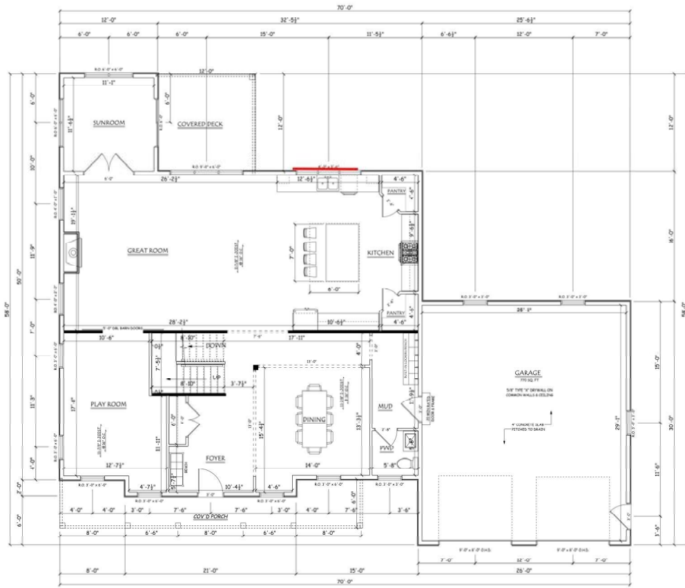
FIRST FLOOR PLAN 8'-0" WALLS 10'-0" CEILING 1'-0" FLOOR FINISH 1'-0" FLOOR FINISH 1'-0" FLOOR FINISH 1'-0" FLOOR FINISH 1'-0" FLOOR FINISH
